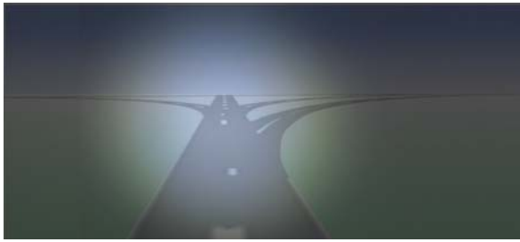
Large portion of the light projected to the road is wasted in traditional DMS because beam shape is symmetrical
